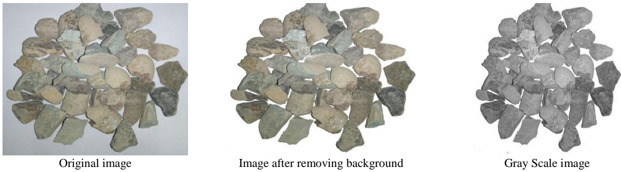
Figure 6. Determination of gray scale of aggregates
